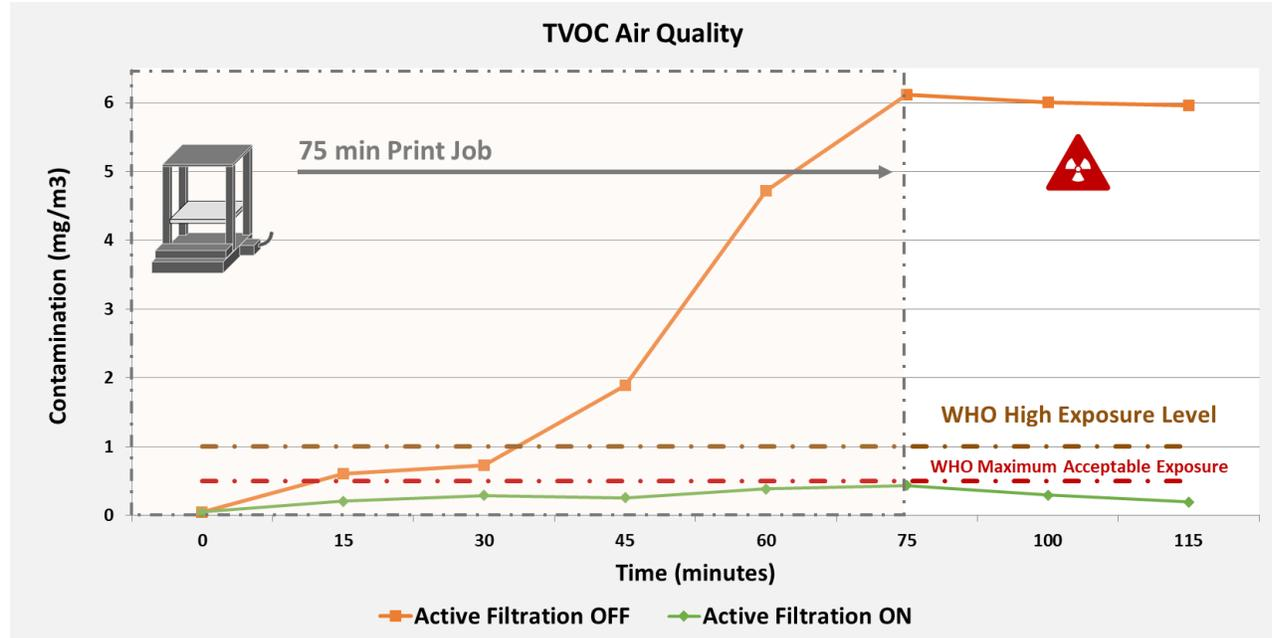
The print without active filtration on for a 75-minute job reached above 6 mg/m<sup>3</sup> which is 2 times the “High” limit and 12 times the “Acceptable” exposure limit provided by the WHO. Using active filtration in the enclosure, the contamination was maintained below 0.45 mg/m<sup>3</sup>
