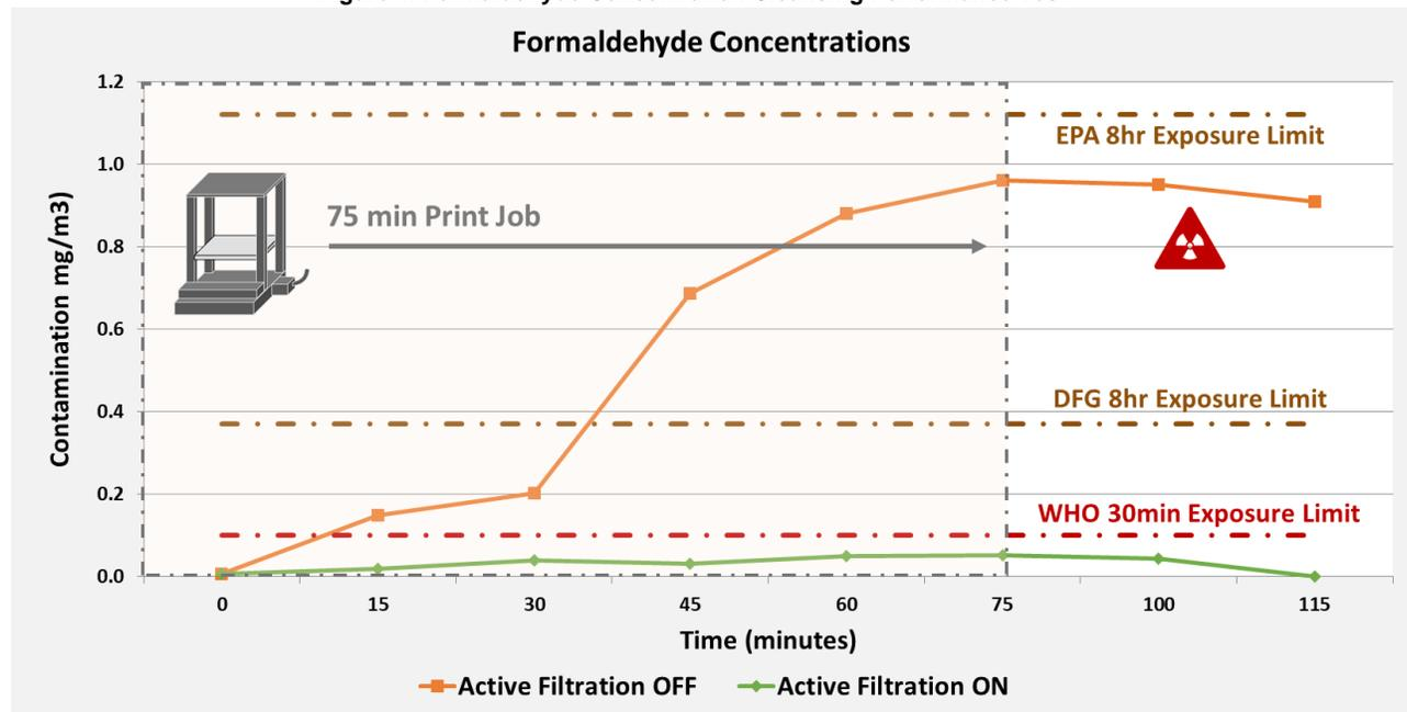
The print without active filtration on for a 75-minute job reached almost 1 mg/m<sup>3</sup> which is more than twice the exposure recommendation by the DFG, almost 10 times that of the WHO and just below the maximum limit set by the EPA. When Active filtration is turned on, the same print stays well below the conservative limitation set by the WHO and goes to nearly ambient formaldehyde concentrations 30 minutes after completion.
