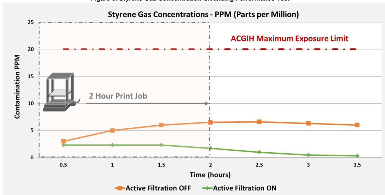
The print without active filtration reached a high of 6.5 ppm which was already below the most conservative of recommendations. Using the active filtration, these numbers were maintained at approximately 2 ppm a 70% reduction and after 1 hour of job completion 0.5 ppm; nearly completely cleaned.
